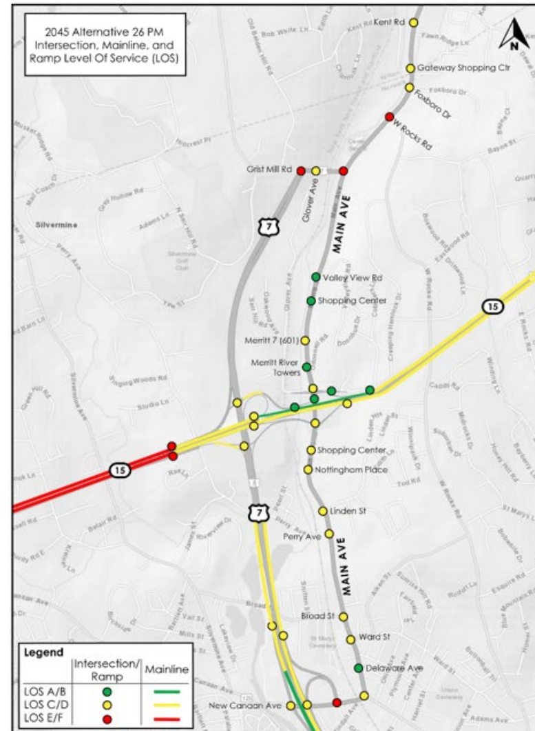
Figure 8.3: Level of Service Summary – 2045 Alternative 26 (AM Peak Hour and PM Peak Hour)
