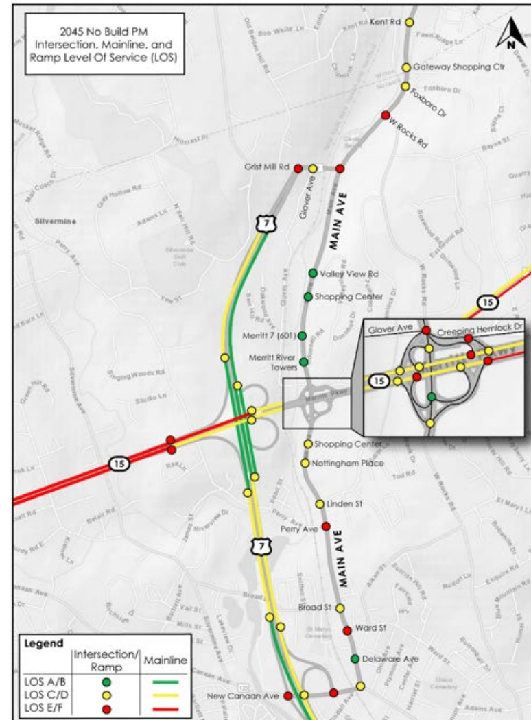
Figure 8.1: Level of Service Summary – 2045 No Build Alternative (AM Peak Hour and PM Peak Hour)
